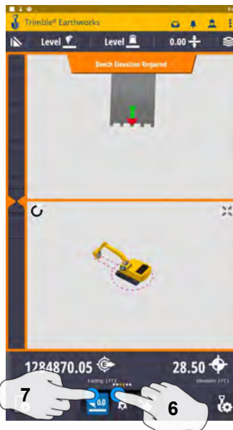
6. Select Blade Tip Focus Point 7. Place Blade Tip at Elevation and Touch Bench
